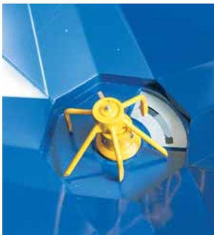
The agitator goes easy on the fertiliser. The small outlet is for small grains and slug pellets.
