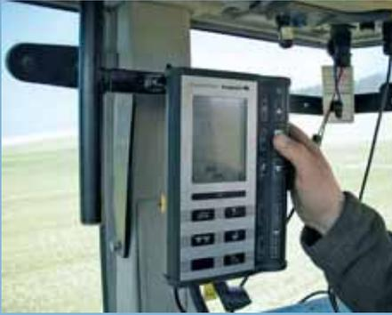
The operation with Calibrator Zurf is simple. The data can be exchanged between PC and the Zurf Terminal using the USB stick.
