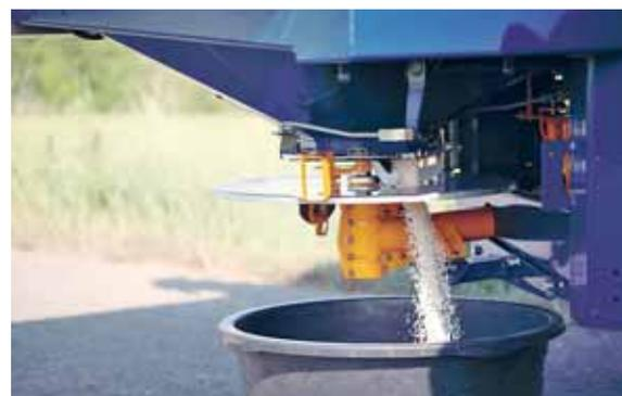
For calibration and emptying of rest quantities there is an opening and a guide plate in the spreading disc.
