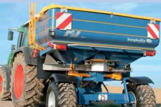
With chassis (€ 3975), also a 60 HP four cylinder tractor is enough for spreading. The speed measurement is non-slip, the attachment and detachment speedy.
