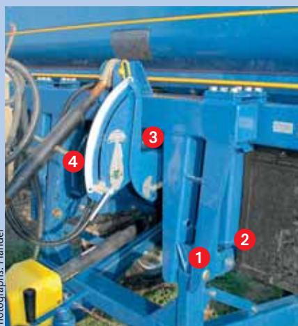
Between the parallel running frames (1)+(2) is the weighing cell (3). The system works exactly. Also good: the scale shows the current slider position (4).
