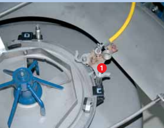
With border spreading from the border, the claw – here the reinforced model (1) – keeps the right slide closed. In our case a too labile compensator was attached.
