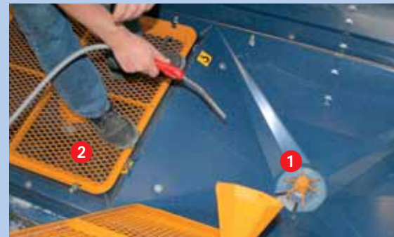
The stirring equipment (1) with an eccentrically rotating star works gently and still effectively. Important: don't forget the grease nipple. The cover grade (2) now lies better in the tank.
