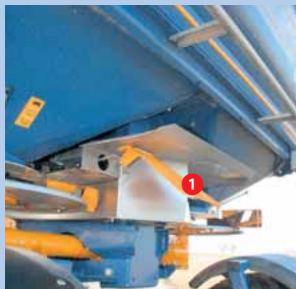
Only with border spreading from the border, in addition a small shield (1) is folded up via servo motor so that more fertilizer is placed on the right.
